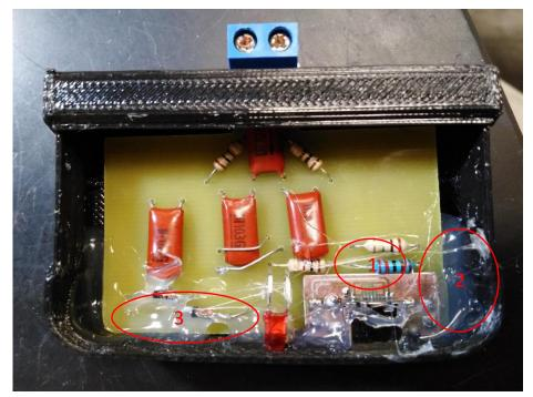
Now put the top part on and fit properly. At last, put in the rivets of size  $\phi 1.7*3$  and use solder to push these rivets a bit deep in the casing. This way the rivets will fit firmly.
