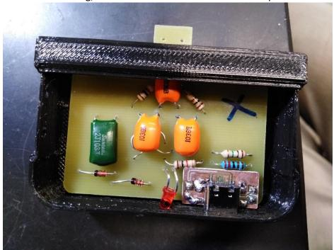
Now push the PCB a little bit so that the USB fits in its slot in the casing. Also adjust the LED in the slot. Now it will look like:
