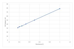
PhysLock output in mV when input signal is changed using Resistance in a voltage divider circuit.
