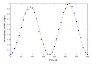
Verifying Maus Law: Intensity of an optical beam as a function of angle between laser source and analyzer, with a current type photodiode at a chopper frequency of 1 kHz, Time Constant: 1 s, I-V converter gain of 1 M, Input Gain: 1x, Reference Phase (Coarse): 1nF, Wavelength of Laser: 405 nm.
