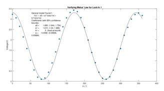
Verifying Malus Law with PhysLock with Time Constant: 1 s, Input Gain: 1x, Reference Phase (Coarse): 1nF, Frequency of Optical Chopper: 1 kHz, Wavelength of Laser: 405 nm.
